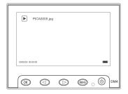
As shown in the figure, enter the Playback mode to view pictures and video files, view the pictures selected by pressing the OK key to view; View the video by pressing the OK key for play/pause; View the current picture/video file, you can press the Up/Down selection key to turn the page, or short press the Menu button again, you can return to the previous level to re-select the file you need to view. -11-
